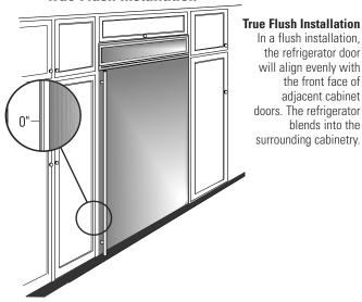
Monogram built-in refrigerators and freezers can be installed flush with typical 24-3/4" deep cabinetry.
